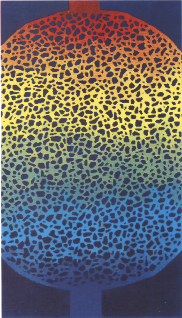
Fig. 3. Pressure distribution for flow through porous media. The dark blue represents the sandstone, the left side (red) is the high-pressure region, and the right side (blue) is the low-pressure region. The sandstone is digitized from a micromodel. The measurement of the permeability for this geometry is about 5% error compared with experimental measurement.
